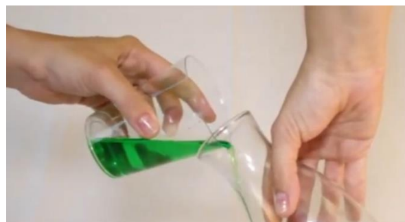
Pouring a liquid down the side of your container.
